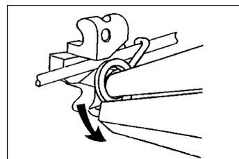
**Figure 2.** As the leg of the spring is withdrawn from the vertical slot, the pliers are rotated toward the arm for easy removal.
