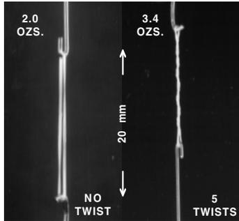
**Figure 2.** Untwisted  $\frac{5}{16}$ " light elastic (left) pulls 2.0 ozs. when extended 20 mm. When twisted 5 times, pull increases to 3.4 ozs. (right).
